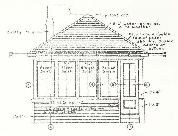
Figure 70. This lookout house was drawn in R-6 in 1934. It has a hipped roof, four light windows and a 14 feet square floor plan.
